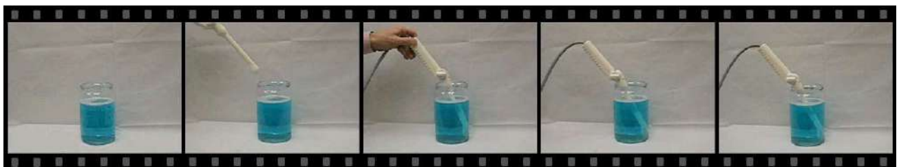
Placing transducer in cleaning solution
