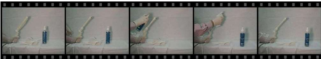
Removing cover and cleaning transducer
